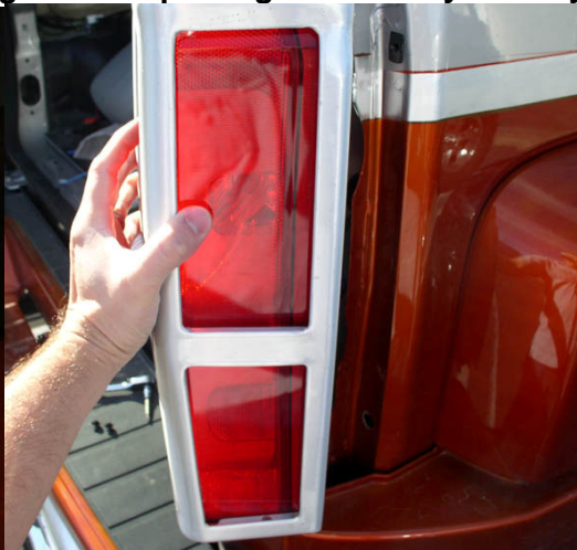
figure 4 snap taillight assembly to body
